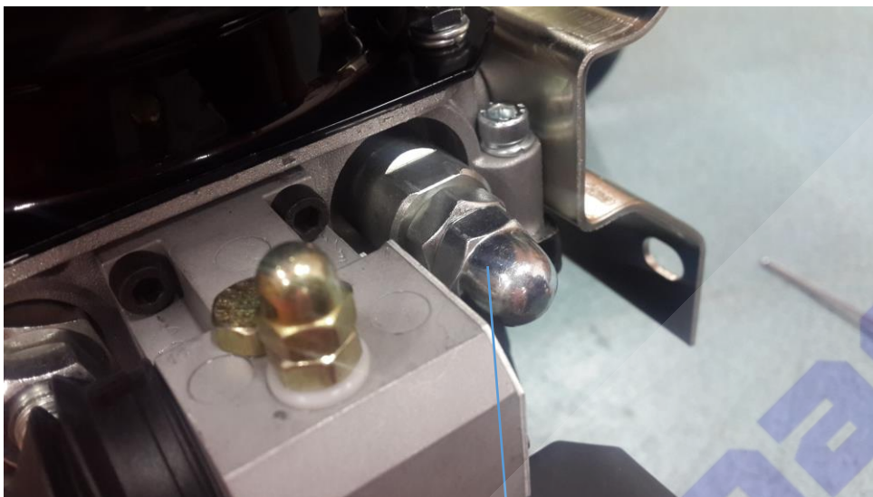
Photo 7. Pressure relief valve
