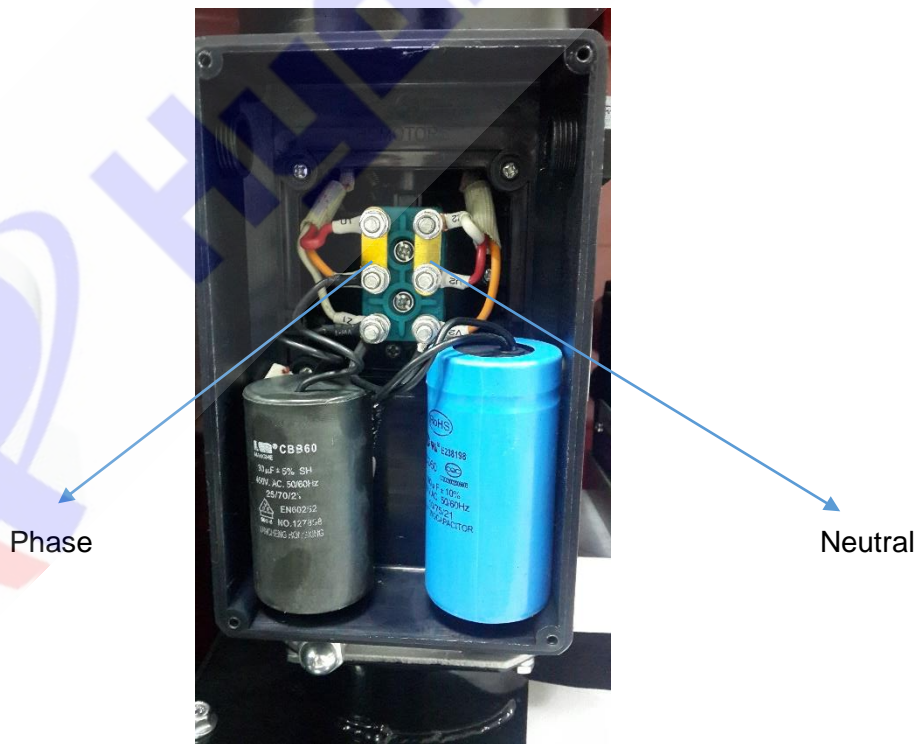
Photo 5. Connection on 220 V AC mono phase motors*
